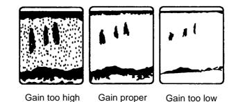
Examples of proper and improper gain levels
